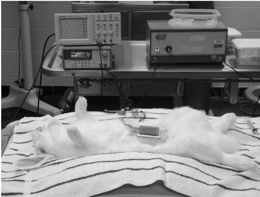
Figure 3 Experimental set-up of the rabbit, 3 \times 3 cymbal array, and electronic drive system during the noninvasive transdermal insulin delivery experiments. With the rabbit anesthetized and lying in the dorsal recumbent position, the waveform generator provided a pulsed signal at 20 kHz, pulse duration of 200 msec, and a pulse repetition period of 1 sec (20% duty cycle). The input peak-to-peak voltage and amplifier gain were adjusted to supply an acoustic I_{SPTP} output of 100 \text{ mW/cm}^2 through the 60 min exposure.
